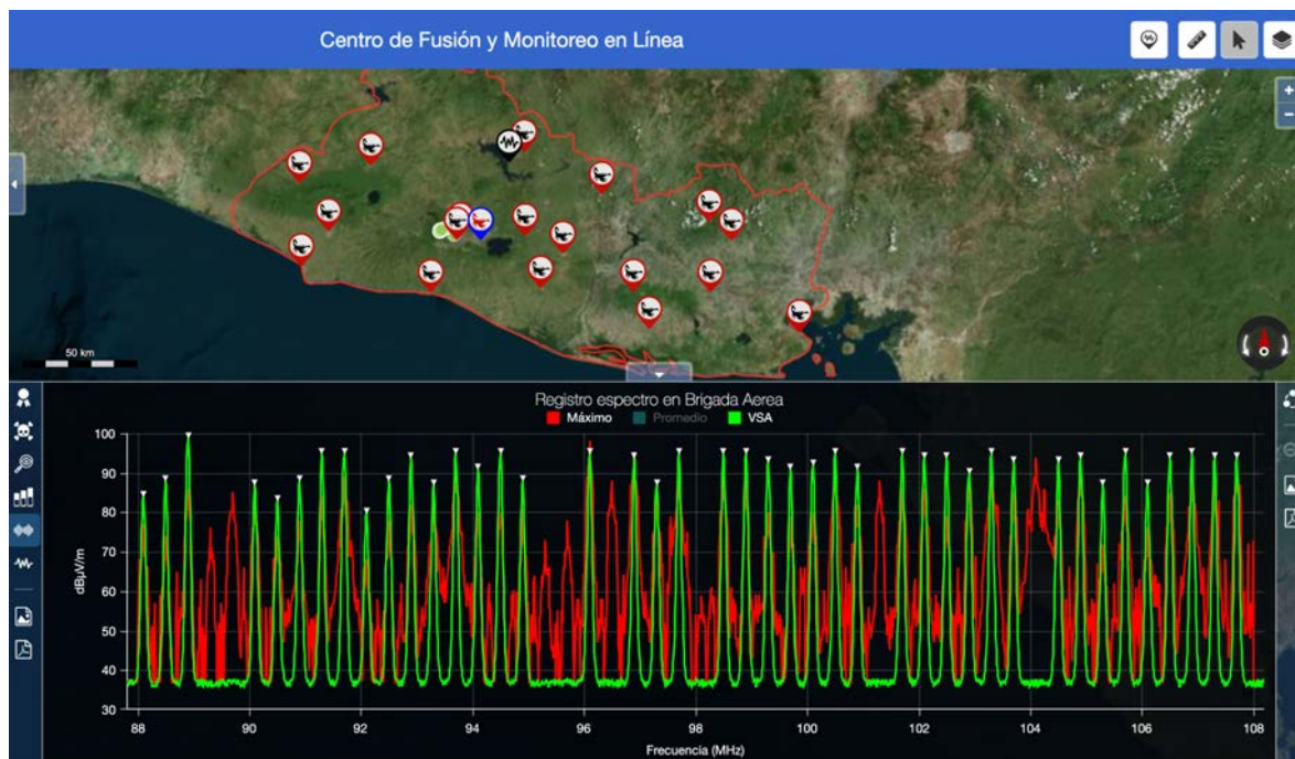
Illustration 6. Automatic Detection of Discrepant FM broadcasting Emissions 5
